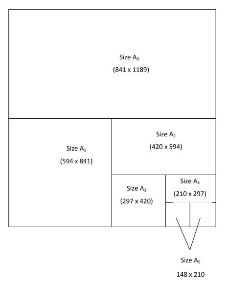
Figure 2: Standard size of drawing sheets according to I.S.I
