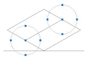
7. Join the line intersection point to intersection point & delete the circle
