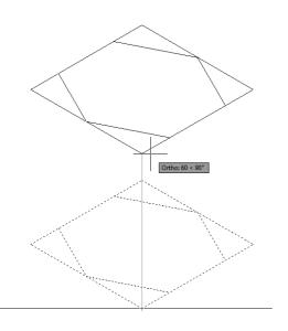
9. Then join the line endpoint to endpoint
