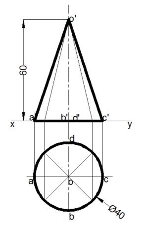
10. Then text & dimension commands are used to obtain the required plan and elevation as shown below.
