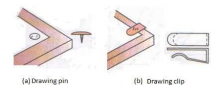
Figure 9 Drawing pins and Drawing clips
