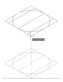
11. Join line from end point to end point
