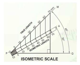
The isometric scale is used to measure the foreshortened length of dimensions of any object to draw the isometric projection. The steps of construction of isometric scale are given below;
