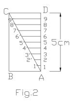
**Problem 2:** On a building plan a line 10cm long represents a distance of 5m. Construct a diagonal scale for the plan to read up to 6m, showing metres, decimetres and centimetres. Indicate the lengths 3.35m and 5.78m on the constructed scale.
