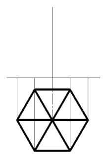
9. Join the line end point to end point & stretch the centre line
