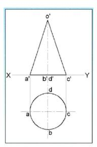
PROJECTION OF SOLIDS WHEN ITS AXIS PERPENDICULAR TO ONE REFERENCE PLANE AND PARALLEL TO THE OTHER
