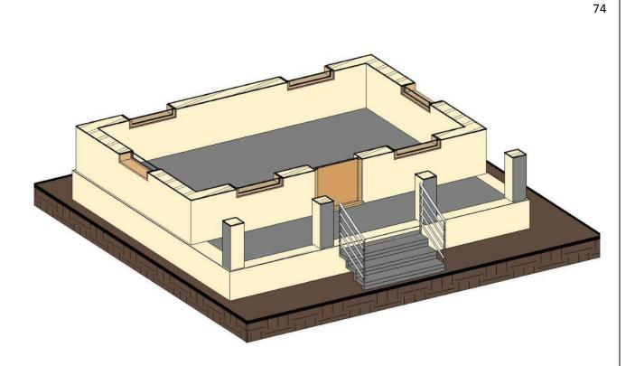
Fig 2. PICTORIAL VIEW OF THE REMAING PORTION OF THE BUILDING CUT BY A HORIZONTAL PLANE JUST ABOVE THE WINDOW SILL LEVEL
